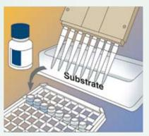
Add 100µl substrate to each well and incubate the wells for 30 minutes
