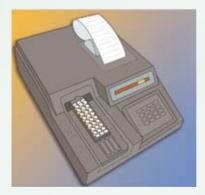
Read wells with a microwell reader using a 450nm filter with a 630nm differential filter and interpret results
