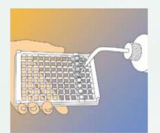
Discard contents from the wells. Wash the wells four times using de-ionized water for pet food or wash solution for wheat gluten.
